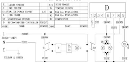
Note: the part in dotted line box is not applicable to some types. Please refer to the real object for the wiring circuit.
